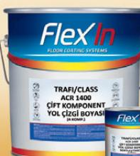
It is a methyl methacrylate based, two component, matt appearance and cold applied road marking paint. Such as pedestrian crossings and speed breakers, etc. used in places. It can be applied in 2 mm or 3 mm thickness. After mixing the products, it should be applied within 7 minutes.
